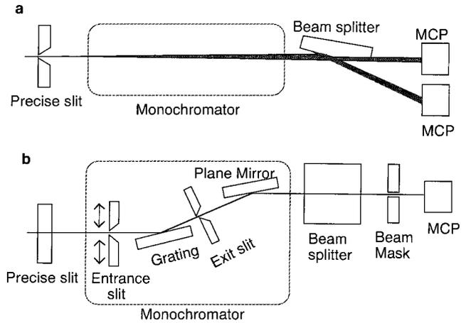
FIG. 2. Optical setup of the two-photon correlator for soft-x-ray synchrotron radiation. (a) is the top view and (b) is the side view. MCP's (microchannel plates) are the fast-response photon detectors with a response time of about 1 ns.
