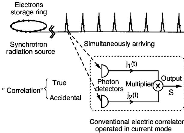
FIG. 1. Illustrating the creation of accidental correlation.  $j_1(t)$  and  $j_2(t)$  are the induced photoelectric currents and  $S$  is the correlation output completed by a linear multiplier.
