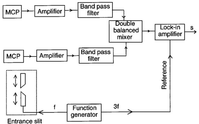
FIG. 3. An electric correlator for soft-x-ray synchrotron radiation. The entrance slit of the monochromator as is shown in Fig. 2(b) is modulated at a slow frequency  $f$  by a piezoelectric translator, and the  $3f$  component of the output of the double balanced mixer, denoted by  $s$ , is detected with a lock-in amplifier.
