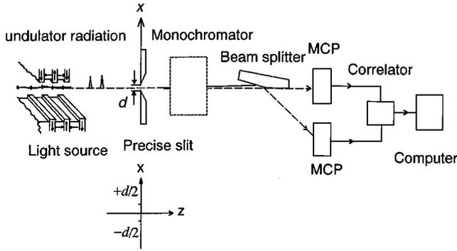
FIG. 4. Top view of the whole experiment system. The light source is the undulator radiation, and the correlation signal is measured as a function of the horizontal width  $d$  of the precise slit that plays a role of the diffraction of the incident synchrotron radiation.
