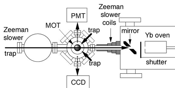
FIG. 2. Experimental setup. The 398-nm laser beams were irradiated to the atoms for the Zeeman slower and the MOT. The fluorescence from the MOT was detected by a CCD camera or a photomultiplier tube (PMT). A mirror with a hole for an atomic beam was set inside a chamber. The right side of the chamber was evacuated with a turbopump, the left with an ion pump.
