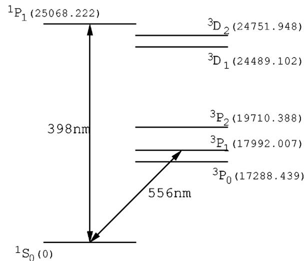
FIG. 1. Energy-level diagram of Yb. The numbers in parentheses represent the energy in  $\text{cm}^{-1}$ . The singlet transition  $^1S_0 \leftrightarrow ^1P_1$  of 398 nm is used for laser cooling. The fluorescence from the  $^3P_1$  state to the  $^1S_0$  state is detected in the measurement of the branching ratio.
