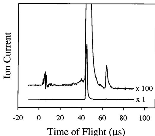
FIG. 1. Time-of-flight spectrum of the detected ions averaged for 200 shots. A large atomic ion signal is observed at  $45.0(2) \mu\text{s}$  after the photoionization pulse. The molecular ion signal observed at  $63.8(2) \mu\text{s}$  corresponds to about three molecules per shot. In these data, the MOT beams were turned off  $0.5 \text{ ms}$  before the photoionization pulse. The small oscillation at  $5 \mu\text{s}$  is due to an electrical transient.
