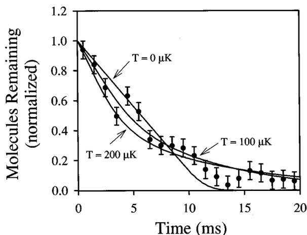
FIG. 3. Relative ion signal arising from cesium dimers as a function of the delay time after the MOT laser beams were turned off. The three solid curves are results from a Monte Carlo simulation. The temporal decay of the signal corresponds to a cesium dimer temperature of about  $100 \pm 100 \mu\text{K}$ .
