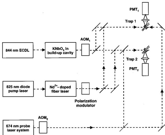
FIG. 2. Overall schematic of the probe and cooling laser system. The acousto-optic modulators (AOM<sub>1</sub> and AOM<sub>2</sub>) switch the cooling and probe lasers off for both traps. The fiber laser output is also polarization modulated and the probe laser system is shown in detail in Fig. 3.
