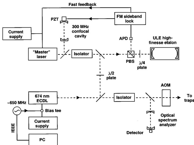
FIG. 3. Detailed arrangement of the 674-nm probe laser system. The master laser has been described previously [2], although the sideband injection locked system has only recently been implemented [12].
