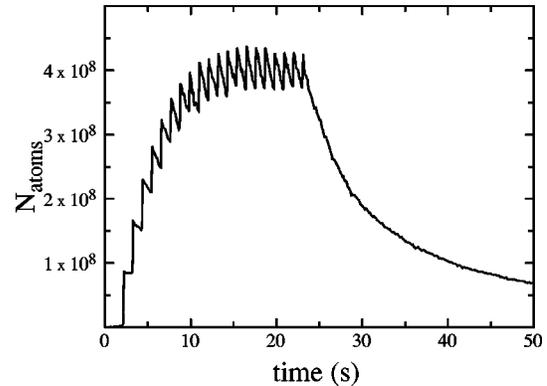
FIG. 2. Fluorescence from MOT<sub>2</sub> as a function of time monitored with a photodiode. Every second during the first 25 s atoms are transferred from MOT<sub>1</sub> and accumulated. For the last 25 s the transfer is stopped and the fluorescence decays following a double exponential.
