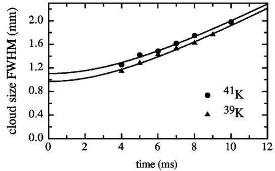
FIG. 3. Free expansion of a cloud of cold atoms after the release from the MOT<sub>2</sub> in the “compressed” phase. Data are taken imaging with a CCD camera the fluorescence of the atoms illuminated, during the expansion, for 100  $\mu\text{s}$  with resonant laser light. The fitted curves give a temperature of 143  $\mu\text{K}$  for  $^{41}\text{K}$  and 136  $\mu\text{K}$  for  $^{39}\text{K}$ .
