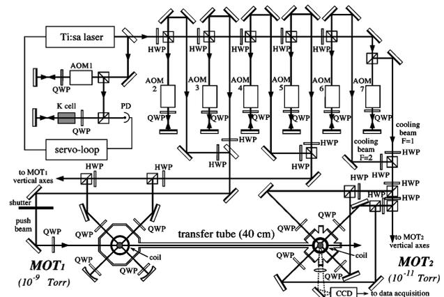
FIG. 1. Experimental apparatus of the double-MOT system for potassium isotopes. Ti:sa, titanium sapphire laser; QWP, quarter wave plate; HWP, half wave plate; AOM, acousto-optic modulator; PD, photodiode. Lenses are not shown for clarity.
