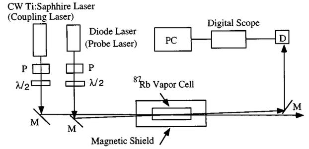
FIG. 2. Experimental arrangement for observation of CPT in Doppler-broadened, multilevel degenerate, open  $^{87}\text{Rb}$  systems.  $P$ 's, polarizers;  $\lambda/2$ 's, half-wave plates;  $M$ 's, mirrors;  $D$ , photodiode detector; PC, personal computer.
