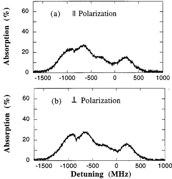
FIG. 6. Measured probe absorption spectra versus the probe laser detuning from the  $F=2 \leftrightarrow F'=2$  transition with a circularly polarized coupling laser tuned to the center of the  $F=2 \leftrightarrow F'=2$  transition. (a) The probe laser was linearly polarized in the  $x$  direction. (b) The probe laser was linearly polarized in the  $y$  direction.
