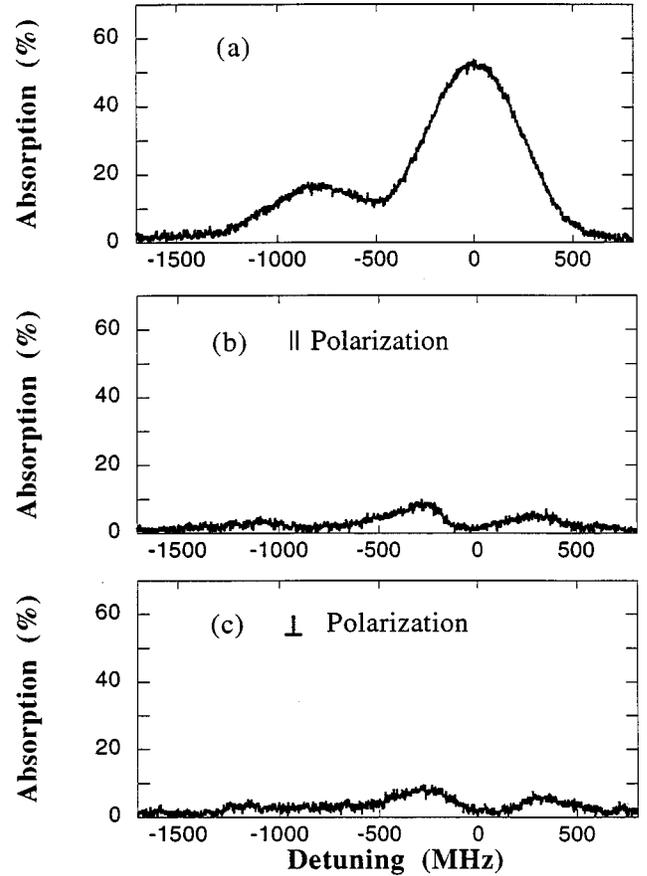
FIG. 7. Measured probe absorption spectra versus the probe laser detuning from the  $F=1 \leftrightarrow F'=2$  transition. (a) The probe absorption spectrum when the coupling laser was blocked. (b) and (c) show the probe spectrum with a linearly polarized coupling laser tuned to the center of the  $F=1 \leftrightarrow F'=2$  transition. (b) The probe laser was linearly polarized parallel to the coupling laser. (c) The probe laser was linearly polarized perpendicular to the coupling laser.
