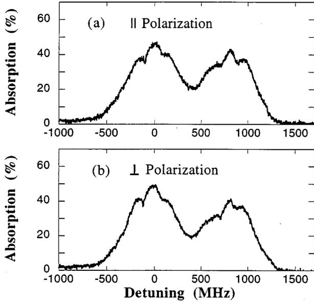
FIG. 4. Measured probe absorption spectra versus the probe laser detuning from the  $F=2 \leftrightarrow F'=1$  transition with a circularly polarized coupling laser tuned to the center of the  $F=2 \leftrightarrow F'=1$  transition. (a) The probe laser was linearly polarized in the  $x$  direction. (b) The probe laser was linearly polarized in the  $y$  direction.
