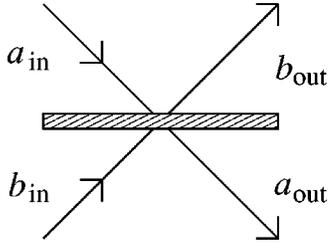
FIG. 1. Schematic drawing of a beam splitter. The incoming modes  $a_{in}, b_{in}$  are piloted into the outgoing modes  $a_{out}, b_{out}$  according to the beam-splitter relations.
