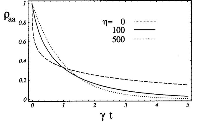
FIG. 6. Time dependence of excitation in spatially homogeneous, dense two-level medium. Time is in units of the inverse free-space decay rate.  $\eta \equiv N\lambda^2 d = 0$  (dotted), 100 (solid line), 500 (dashed line).  $g = \gamma/\sqrt{2\pi}\Delta_D = 0.01$ .
