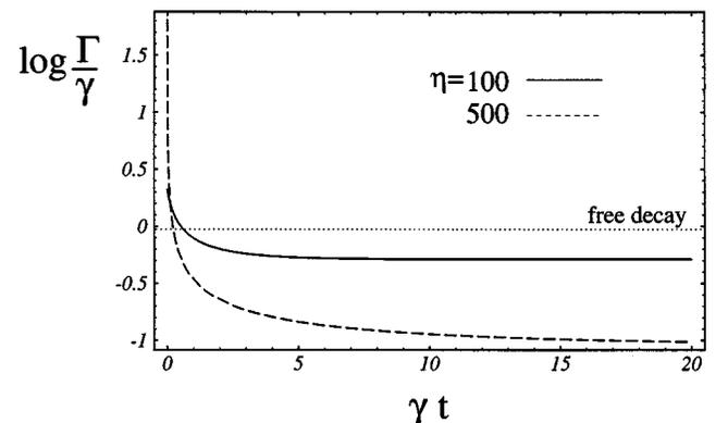
FIG. 7. Effective rate of decay  $\Gamma_{\text{eff}} = -\dot{\rho}_{aa}/\rho_{aa}$  for examples of Fig. 6. Dotted line corresponds to free-space decay. Amplified spontaneous emission in the initial phase and slowdown of decay in final phase are apparent.
