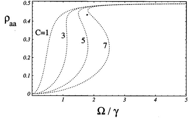
FIG. 10. Stationary excited-state population as function of driving-field Rabi-frequency  $\Omega$  for different cooperativity parameters. Here,  $\Gamma = \gamma^* = 0$ .
