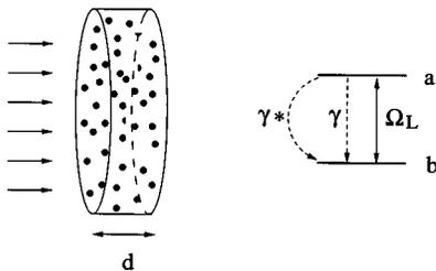
FIG. 9. Strongly driven, dense two-level medium.  $\gamma$  and  $\gamma^*$  describe radiative and nonradiative decays, respectively, and  $\Omega_L$  denotes Rabi frequency of local field.
