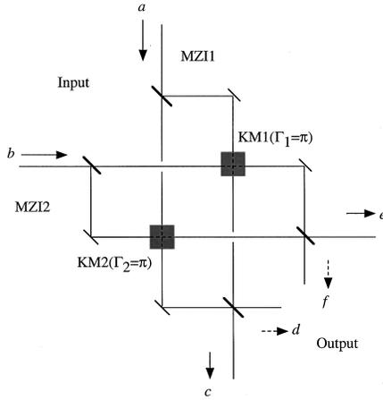
FIG. 3. Configuration of our proposed nonlinear optical gate (NOG). KM, optical Kerr medium; MZI, Machzehnder interferometer.
