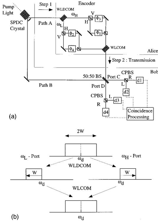
FIG. 2. (a) Modified configuration of the quantum communication system with entangled twin photons. (b) Division and recombination of the photon wave packet in the frequency domain via WLDCOM and WLCOM, respectively.
