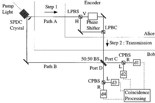
FIG. 1. Basic configuration of a quantum communication system with entangled twin photons. Step 1, sending the signal photon to Alice in advance; step 2, transmitting the signal photon to Bob after encoding information.
