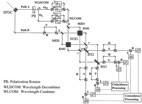
FIG. 4. Modified configuration of the dense coding quantum communication with an enhanced capacity.
