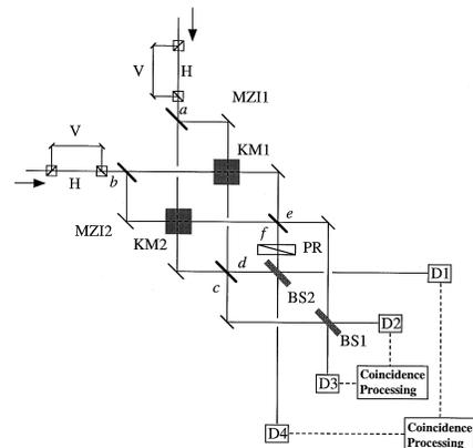
FIG. 5. Simplified configuration of the perfect Bell-state analyzer.
