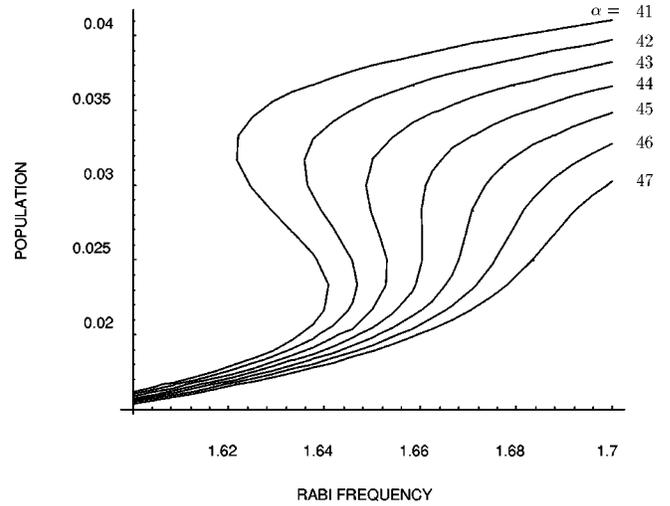
FIG. 2. Results of numerical calculations of Eq. (6) demonstrating the disappearance of the three-valued solution with the annihilation constant  $\alpha$ . Bistability exists at  $\alpha < \alpha_c = 44$  in full correspondence with Eq. (8). The other parameters are  $\Gamma/\Gamma_2 = 2$  ( $\Gamma_1, \Gamma_2 \gg 1$ ),  $\Delta' = -10$ , and  $|\Delta_L| = 100$ . All numbers are in units of  $\gamma_R$ .
