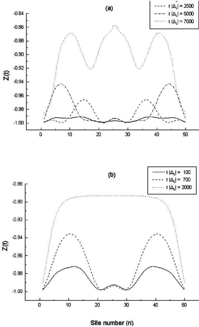
FIG. 6. Spatial distribution of the population difference at several instants in time evolution (shown in the insets). The Rabi frequency is equal to 0.645 (a) and 0.861 (b). The other parameters are the same as in Fig. 5.
