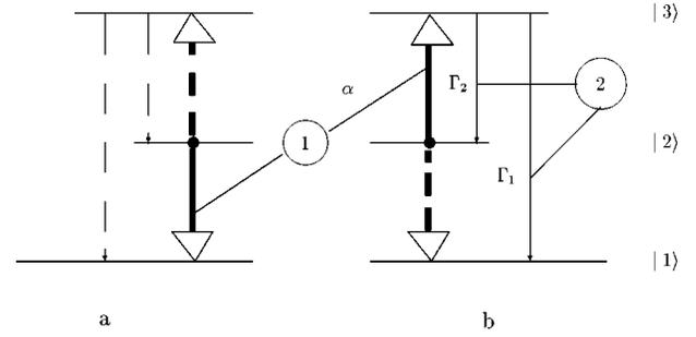
FIG. 1. Scheme of the exciton-exciton annihilation process through a third molecular level. In the first step, the molecule  $a$  goes to the ground state while the molecule  $b$  passes to the third level. The second step is the radiationless relaxation of the third level to the ground and excited states of the transition of interest. Dashed arrows indicate the cross-processes.
