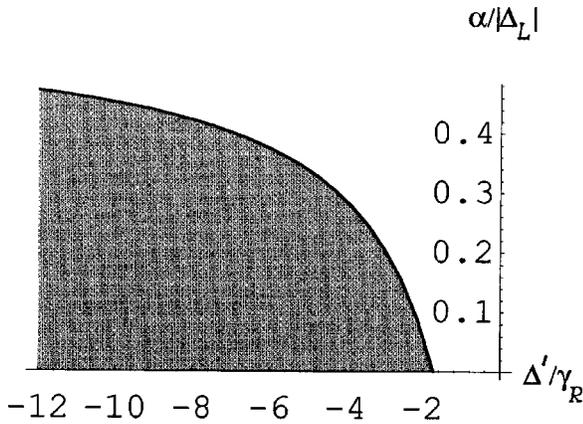
FIG. 3. Dependence of the critical value of the annihilation constant  $\alpha_c$  on the initial resonance detuning  $\Delta'$ . The shaded part corresponds to the existence of aggregate bistability [ $\alpha < \alpha_c(\Delta')$ ].
