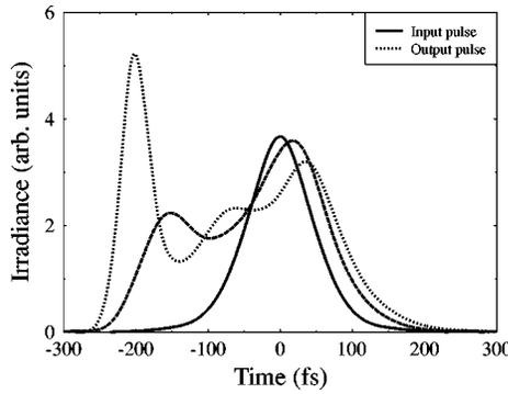
FIG. 6. Pulse irradiance profiles for propagation through the semiconductor amplifier at the gain peak; strong pulse reshaping occurs as a manifestation of amplification and adiabatic following (see the text).
