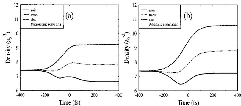
FIG. 5. (a) Temporal behavior of the total electron-hole density for the microscopic scattering processes for excitation in the gain (solid line), transparency (dotted line), and absorption regime (dashed line) of the SOA. The input Rabi energy was 50 meV. (b) Same as in (a), but by employing an adiabatic elimination for the polarization equation (see the text).
