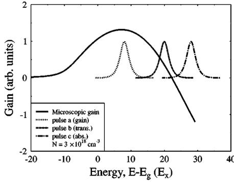
FIG. 1. Gain spectrum for a semiconductor amplifier at room temperature with an incoherent electron-hole density of  $N=3 \times 10^{18} \text{ cm}^{-3}$ . Also shown are the spectral profiles of the incident pulses ( $\tau_p=120 \text{ fs}$ ) excited in the gain, transparency, and absorption regimes of the SOA. Energy is in units of excitonic binding energy ( $E_x$ ).
