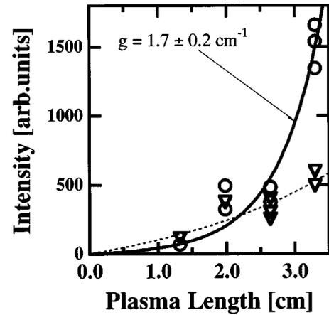
FIG. 3. Intensity of the  $154.7\text{-\AA}$  Li-like Al laser ( $\circ$ ) and the  $141.7\text{-\AA}$   $4p-3s$  line ( $\nabla$ ) as a function of plasma length observed at  $300 \mu\text{m}$  from the target surface. The peak intensity of the pump is  $1.04 \pm 0.04 \text{ TW}/\text{cm}^2$ . The lines correspond to the least-squares fitting of each data set to the Linford formula [21].
