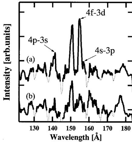
FIG. 2. Time-integrated spectra observed in the on-axis direction, for plasma lengths of (a) 3.3 cm and (b) 2.0 cm. These spectra are observed at  $300 \mu\text{m}$  from the target surface, at a peak pump intensity of  $1.04 \text{ TW}/\text{cm}^2$ .
