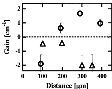
FIG. 4. Small-signal gain coefficient of the 154.7-Å Li-like Al laser as a function of distance from the target surface. The peak intensity of the pump is 1.04 (○) and 0.88 TW/cm<sup>2</sup> (△).
