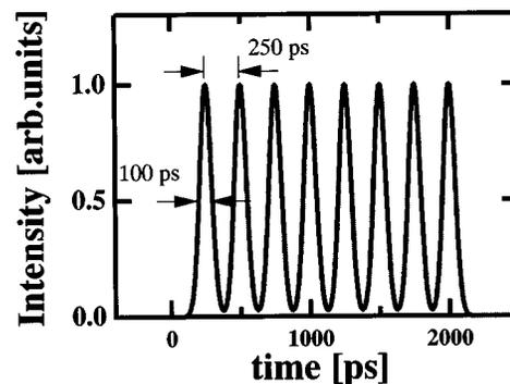
FIG. 1. Typical time history of the multipulse-pump laser intensity at the target surface, for a 3.3-cm-long line focus.
