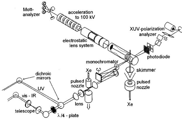
FIG. 1. Experimental setup for photoelectron spin-polarization measurements using VUV radiation, generated by sum-frequency mixing of two laser beams in xenon. In the case of angular distribution measurements the  $\lambda/4$  retarding plate is replaced by a  $\lambda/2$  Fresnel rhomb to rotate the plane of linear polarization of the light and the Mott polarimeter and electrostatic lens system is replaced by a double multichannel plate for photoelectron yield detection.
