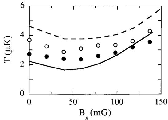
FIG. 4. Kinetic temperature  $T$  vs transverse field  $B_x$ , for parallel fields  $B_z=0$  mG (filled circles), and  $B_z=90$  mG (open circles), respectively. Solid and dashed lines are the corresponding QMCWF simulations. Lattice parameters are  $U_P=108E_R$  and  $\Delta=-21\Gamma$ .
