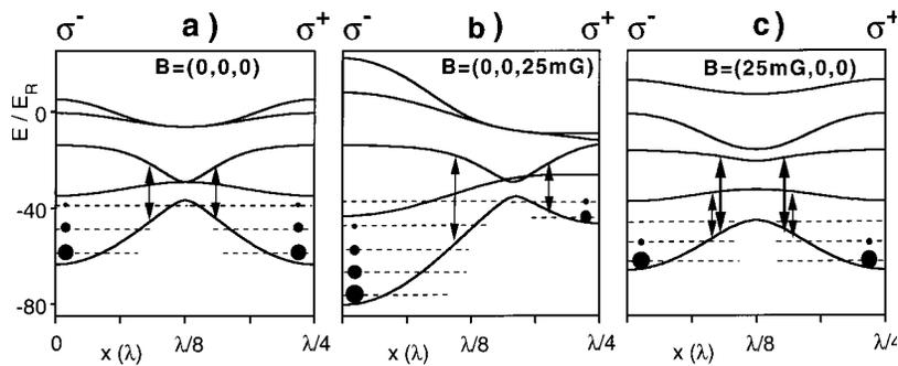
FIG. 2. Adiabatic lattice potentials for (a) no magnetic field, (b) longitudinal magnetic field, and (c) transverse magnetic field. The modulation depth of the  $m = \pm F$  diabatic potential is  $U_P = 70E_R$ , and the lattice detuning  $\Delta = -20\Gamma$ . For simplicity we show potentials for  $F = 2$ ; the arguments in the text apply for  $F \geq 2$ . Dashed lines and dots indicate vibrational states and their population; the arrows indicate Raman- and magnetically induced mixing.
