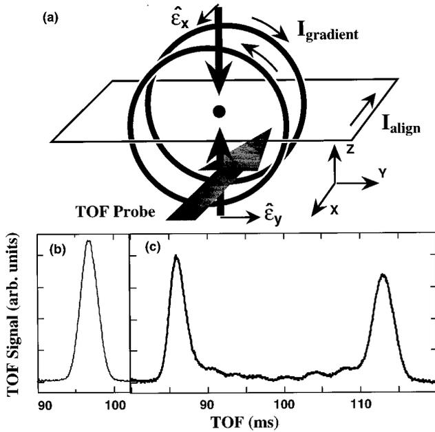
FIG. 1. (a) Experimental setup for TOF measurements. A pair of coils in the anti-Helmholtz configuration provides the magnetic-field gradient for Stern-Gerlach analysis. The square coil provides a bias magnetic field to maintain alignment of the atomic spin. (b) Typical TOF distribution without field gradient. (c) Typical TOF distribution with magnetic-field gradient. The states  $|m = -4\rangle$  and  $|m = -3\rangle$  are not resolved; we account for this in our fitting procedure.
