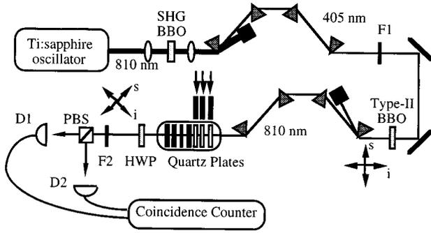
FIG. 1. Schematic of the experimental setup. SHG is a frequency-doubling crystal, F1 and F2 are interference filters, HWP is a half-wave plate oriented to rotate the polarizations of the down-converted photons by  $45^\circ$ , PBS is a polarization beam splitter, and D1 and D2 are avalanche photodiodes.
