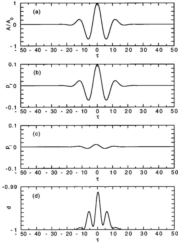
FIG. 4. Solutions for a cosinusoidal-Gaussian input pulse with the same parameter values as Fig. 1, except that the pulse amplitude is here reduced from  $A_0=10.0$  to  $A_0=1.0$ , the width is increased from  $\tau_0=1.0$  to  $\tau_0=10.0$ , and the frequency is reduced from  $\omega'=5$  to  $\omega'=0.5$ . In contrast to Fig. 1, the polarization components are both in phase with the field.
