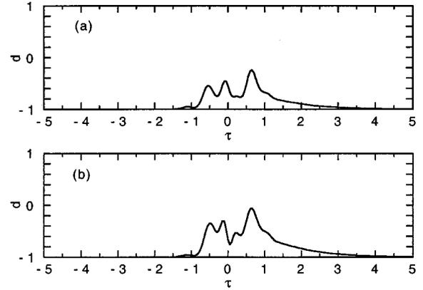
FIG. 2. Population difference solutions for nonzero values of the dipole moment difference  $\mu_d$  including (a)  $\mu_d=0.2$  and (b)  $\mu_d=0.5$ . In these cases the population difference has higher harmonics of the underlying field frequency.
