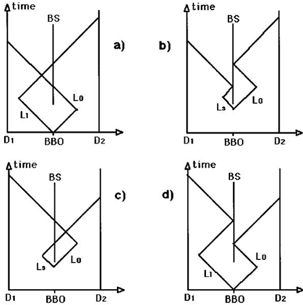
FIG. 5. (a) and (b) are two amplitudes to detect a photon pair such that  $D_1$  fires ahead of  $D_2$ ; (c) and (d) are two amplitudes to get a detection in the reversed order.
