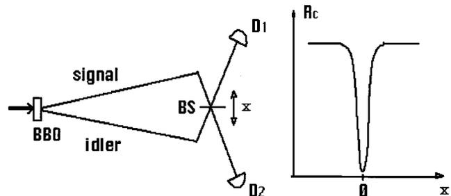
FIG. 1. Typical two-photon interferometer. The signal and idler from spontaneous parametric down-conversion are mixed by a beam splitter BS and detected by detectors  $D_1$  and  $D_2$  for coincidences.
