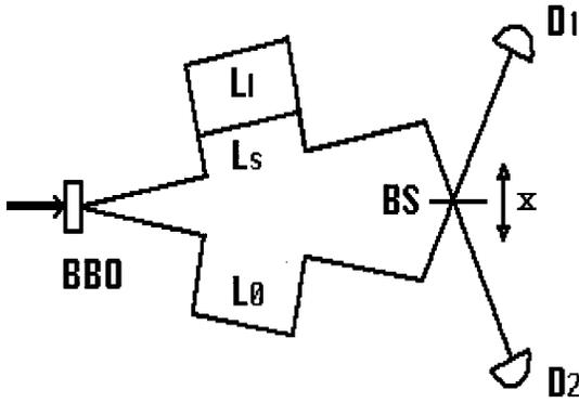
FIG. 2. Scheme of our experiment. In contrast with Fig. 1, there are two optical paths  $L_l$  and  $L_s$  in the signal beam. The idler path length is  $L_0$ .
