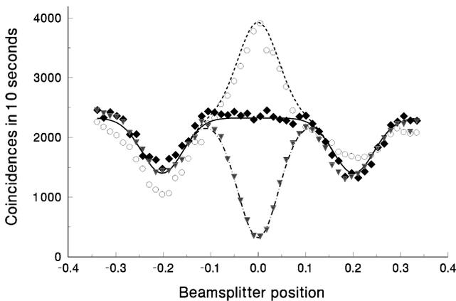
FIG. 3. Observed coincidence counting rate as a function of the beam-splitter position (in millimeters). The triple dip-peak pattern corresponds to different phases  $\phi=0, \pi/2$ , and  $\pi$  (triangles, diamonds, and circles, respectively). The side dips do not change significantly, while the central part changes from dip to peak. The raw data are fitted according to the theoretical predictions of Eq. (5).
