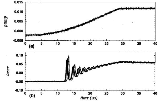
FIG. 2. FPT measurements with slowly swept pump. The pump power (a) is ramped up slowly with respect to the period of oscillations of the laser dynamics at turn-on (b). Pump and laser intensity units are arbitrary. 15 overlaid traces of both the pump and intensity are depicted. Maximum pump power is 1.0 W. Laser gas pressure is  $30\ \mu\text{bar}$ .
