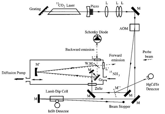
FIG. 1. Experimental setup.  $L$ : ZnSe lenses focus the pump beam through the acousto-optic modulator (AOM);  $M$ : flat mirror;  $M'$ : 2.0 m ROC movable mirror controls the ring laser tuning;  $M''$ : beam splitter reflects portion of the pump beam to HgCdTe detector;  $G_r$ : grating couples the  $\text{CO}_2$  radiation into the ring resonator (80 lines/mm);  $W_M$ : wire mesh output coupler (5 lines per mm). See text.
