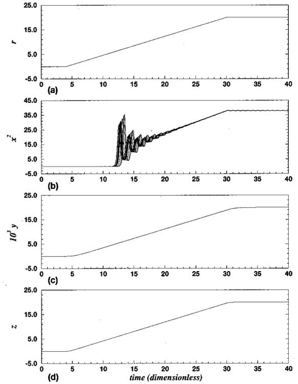
FIG. 3. Intensity (b) calculated from Lorenz equations for slow increase of pump (a) with time (dimensionless—1 unit in the Lorenz system corresponds to  $1 \mu\text{s}$  in the Lorenz-Haken system for the choice  $\gamma_{\perp} = 1$  MHz). 10 traces.  $r_{\text{max}} = 20$ ,  $\epsilon = 1.0 \times 10^{-3}$ . (c),(d): Lorenz-Haken variables  $y, z$  corresponding to small signal polarization and inversion, calculated with  $\dot{x} = 0$  and  $x = 0.001$ . All variables are dimensionless.
