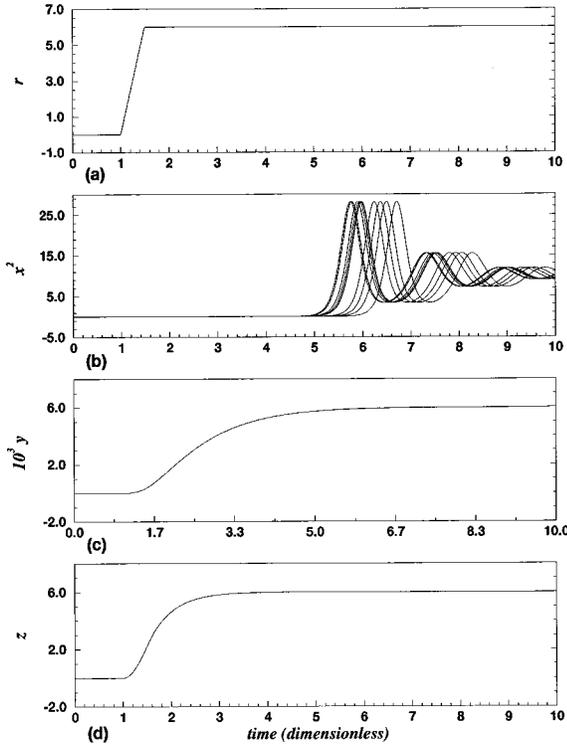
FIG. 5. Intensity (b) calculated from Lorenz equations for rapid increase of pump (a) with time (dimensionless). 10 traces.  $r_{\max} = 6.0$ ,  $\epsilon = 1.0 \times 10^{-3}$ . (c),(d): Lorenz variables  $y, z$  corresponding to small signal polarization and inversion, calculated with  $\dot{x} = 0$  and  $x = 0.001$ . All variables are dimensionless.
