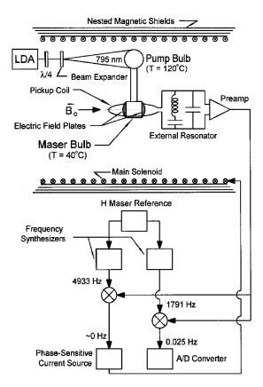
FIG. 1. Schematic diagram of the dual noble-gas maser used to make the measurements reported here. Electric-field plates were not installed in the experiments reported in this paper.
