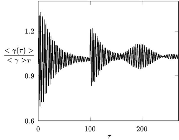
FIG. 1. Numerical simulation of the echo effect discussed in the text,  $\gamma(\tau) = x^2(\tau)$ . The parameters for the simulations are  $\tau_p = 105$ ,  $\xi_1 = 0.2$ ,  $\xi_2 = 0.1$ , and  $\theta = T/4V_0 = 0.03$ .
