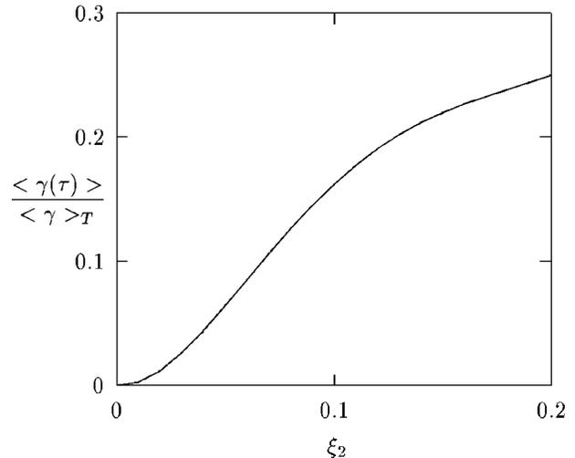
FIG. 2. Maximum echo amplitude as a function of the intensity  $\xi_2$  of the second pulse.
