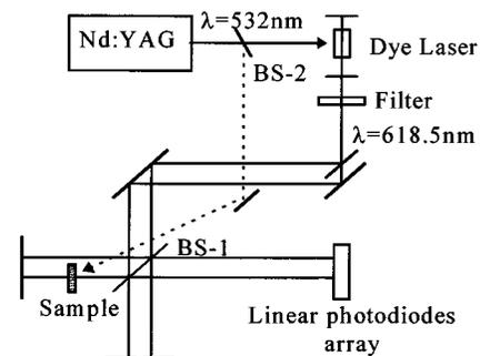
FIG. 1. Experimental scheme used to measure the nonlinear refraction index of the disordered media. For the nondegenerate  $n_2$  measurement a beam splitter BS-2, is introduced to divert the pump beam.
