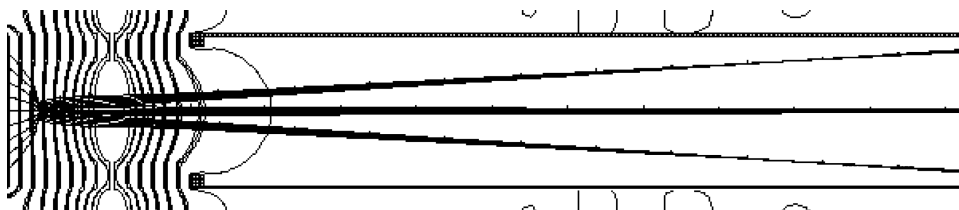
FIG. 3. Field geometry in the recoil-ion–electron spectrometer. The three groups of trajectories result from ions starting with different momenta in the direction perpendicular to the electric field.
