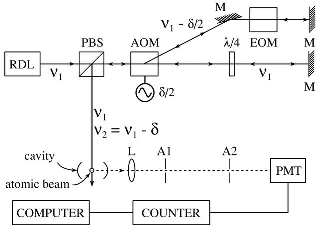
FIG. 2. Experiment schematic: RDL, cw ring dye laser; PBS, polarization beam splitter; AOM, acousto-optic modulator; M, mirror;  $\lambda/4$ , quarter wave plate; EOM, electro-optic modulator; L, lens; A1 and A2, apertures; PMT, photomultiplier tube.
