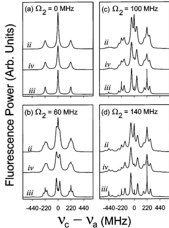
FIG. 5. Traces *iii* (*iv*) represent simulated results for  $\Gamma_c = 2$  MHz (13 MHz) when only a single isotope species is considered. Traces *ii* are the same as in Fig. 3.
