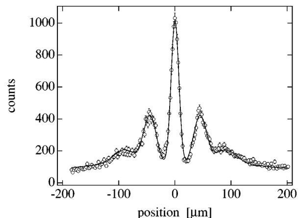
FIG. 5. Diffraction at a purely imaginary potential: far-field diffraction pattern for the scattering of metastable argon atoms at one of the resonant light gratings (801.7 nm). A  $10\text{-}\mu\text{m}$  slit was scanned directly in front of the “channeltron” detector and the spatial atomic diffraction image was recorded as a function of the slit position.
