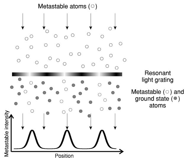
FIG. 1. “Absorption” grating for metastable atoms made by resonant light. Metastable atoms (open circles) are excited by the resonant light and consequently pumped to their ground state (filled circles), which is undetected. Only atoms near the nodes of the light field survive in their original metastable state.
