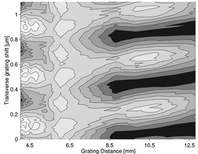
FIG. 4. Atomic wave field behind the first absorptive grating (brighter regions correspond to higher atomic densities). The data were measured, similar to Fig. 2, by scanning the relative spatial phase of the two gratings and recording the total number of transmitted atoms at several distances (from 4 to 13 mm) between the two gratings. A doubling of the spatial period, as expected for the Talbot near-field regime, is observed at a distance of 5.8 mm.
