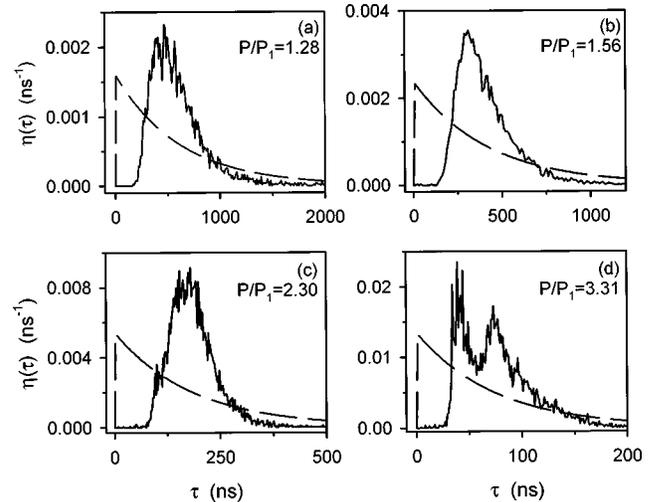
FIG. 2. Observed power dropout time-interval probability densities (solid lines) and the predictions of the HK model (dashed line) for (a)  $\mathcal{I}=18$  mA ( $P/P_1=1.28$ ),  $\Delta\tau=10$  ns; (b)  $\mathcal{I}=19$  mA ( $P/P_1=1.56$ ),  $\Delta\tau=10$  ns; (c)  $\mathcal{I}=22$  mA ( $P/P_1=2.30$ ),  $\Delta\tau=10$  ns; and (d)  $\mathcal{I}=26$  mA ( $P/P_1=3.31$ ),  $\Delta\tau=1$  ns.
