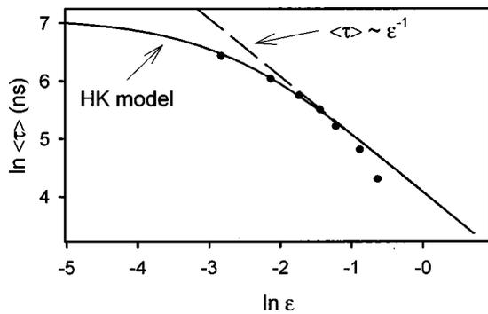
FIG. 4. Mean time interval between power dropout events as a function of  $\epsilon = (\mathcal{I} - \mathcal{I}_{th})/\mathcal{I}_{th}$ . The circles are the observed values, the solid line indicates the predictions of the HK model, and the dashed line indicates the scaling expected for type-II intermittency. Note that one data point for  $\epsilon=0$  cannot be shown on this plot; it agrees well with the HK model.
