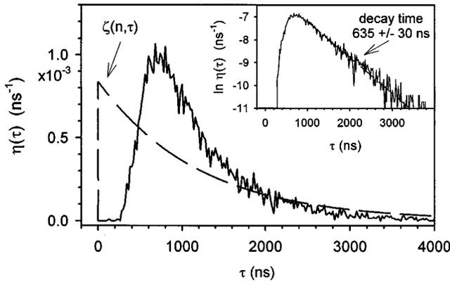
FIG. 1. Observed power dropout time-interval probability density for  $\mathcal{I}=17$  mA ( $P/P_1=1$ ) with  $\Delta\tau=10$  ns (solid line) compared to the distribution predicted by the HK model (dashed line) using the measured value of  $\langle\tau\rangle$ . The inset demonstrates that distribution decays exponentially for long times.
