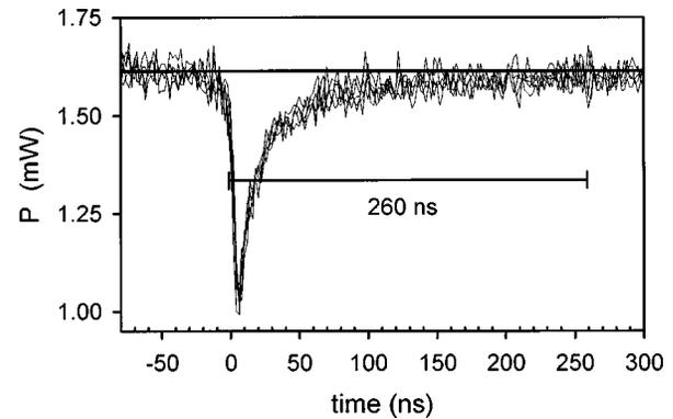
FIG. 5. Temporal evolution of the average laser power for  $P/P_1=1$  during a series of power dropout events, illustrating that they are nearly identical. The length of the dropout event is approximately equal to the dead zone shown in Fig. 1. The analog bandwidth of the detection system for these measurements is 250 MHz.
