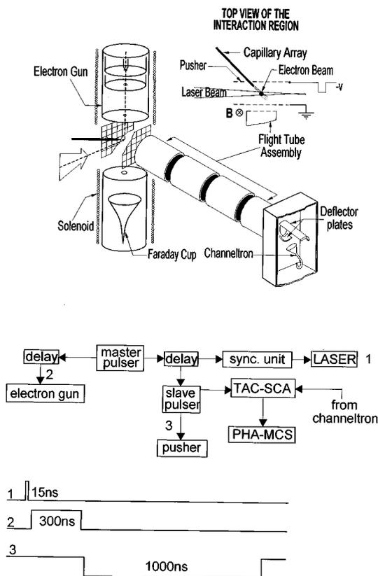
FIG. 1. Schematic of the experimental arrangement. TAC-SCA is time to amplitude converter with single channel analyzer and PHA-MCS is the pulse height analyzer with multichannel scalar.
