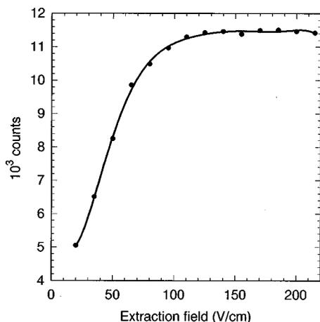
FIG. 2. Number of ions extracted as a function of the extraction field.
