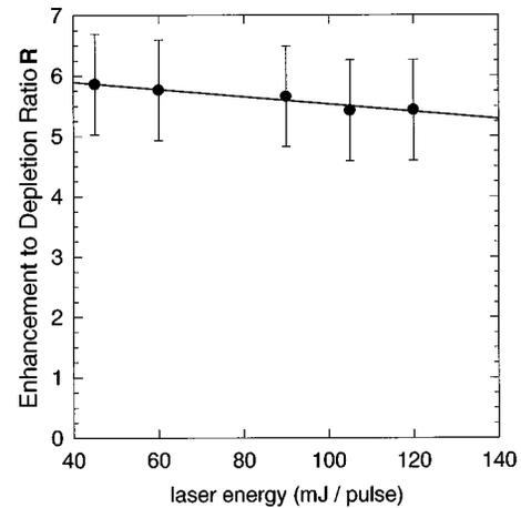
FIG. 5. Ratio  $R$  of the number of  $O^-$  ions formed from the excited state to the reduction in the number of ions from the ground state. The error bars represent the statistical error.
