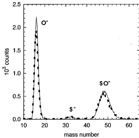
FIG. 4. Time-of-flight spectra of negative ions at the electron energy of 4.6 eV with (dotted line) and without (continuous line) laser excitation.
