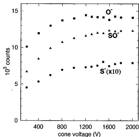
FIG. 3. Number of ions detected as a function of the voltage on the nose cone of the channeltron for negative ions of interest in the present experiment. The voltage across the channeltron is kept constant.
