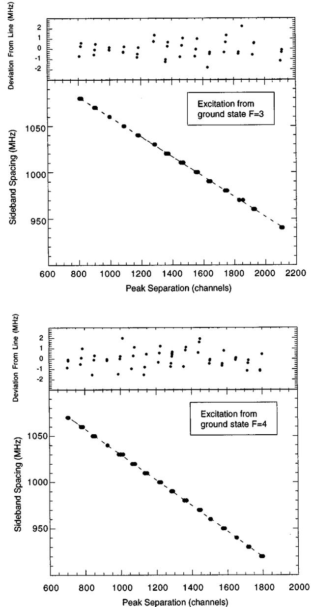
FIG. 4. Separation between  $F'=4$  (zeroth-order sideband) to  $F'=3$  (first-order sideband) laser fluorescence peaks as a function of rf sideband frequency with the residuals to a least-squares linear fit to the data.
