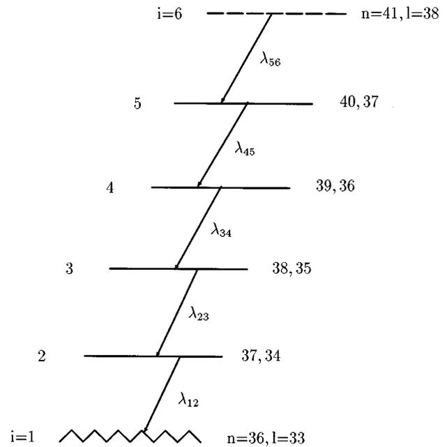
FIG. 1. Part of the energy-level diagram of  $\bar{p}\text{He}^+$ . Solid lines show the metastable states, zigzag line denotes the short-lived annihilation state, dashed line shows the states depopulated by collisions.
