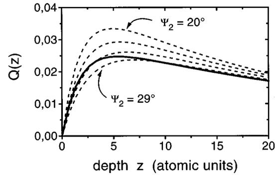
FIG. 4. The depth distributions of *K* Auger emission, according to the two-step model. Solid line:  $E_{\text{ion1}} = 102$  keV and  $\Psi_1 = 20^\circ$ ; dashed lines:  $E_{\text{ion2}} = 51$  keV and  $\Psi_2 = 29^\circ, 26^\circ, 23^\circ,$  and  $20^\circ$  (from bottom to top).
