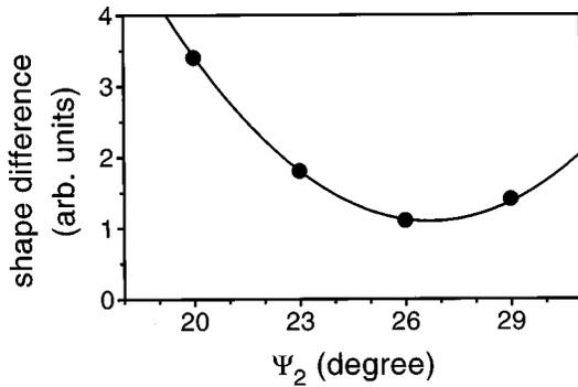
FIG. 3. The measure of difference of shape for the four pairs of corresponding spectra shown in Fig. 2. The line is to guide the eye. The best agreement is obtained about  $\Psi_2 = 26 \dots 27^\circ$ .
