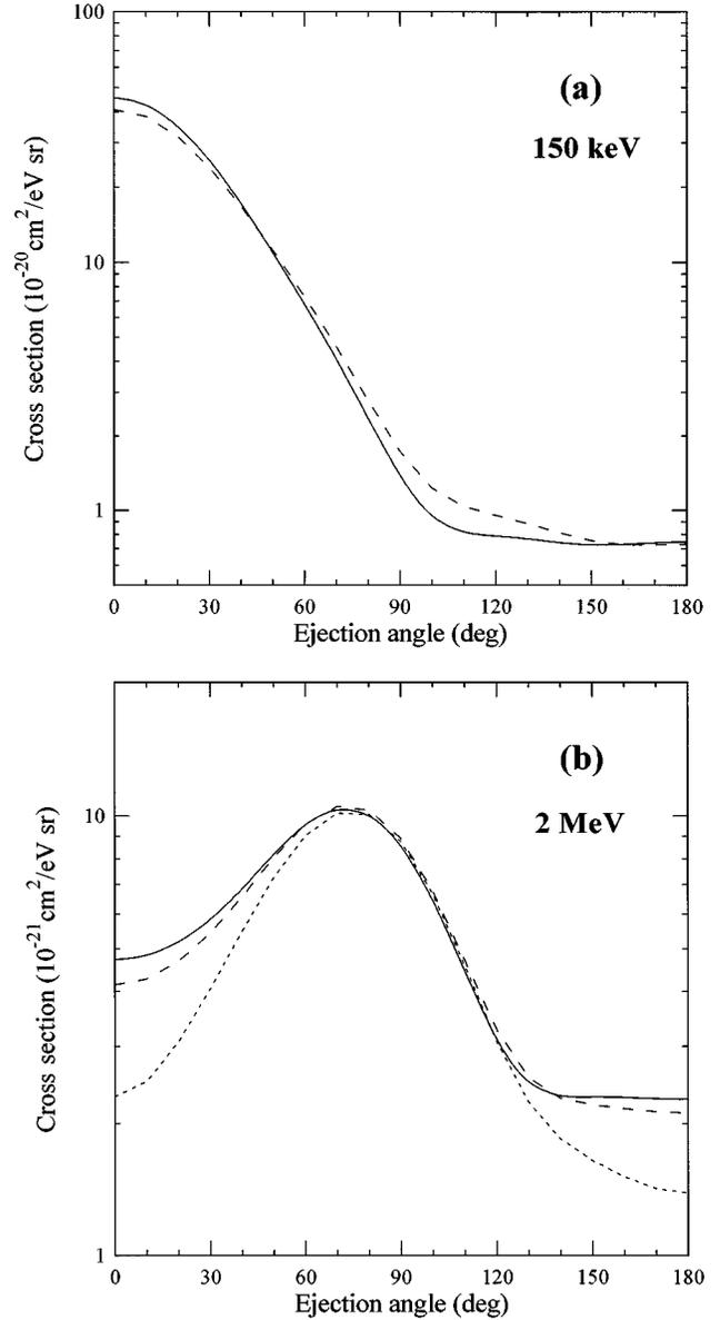
FIG. 3. Ionization cross section for the ejection of a 33-eV electron from He by (a) 150-keV and (b) 2-MeV protons as a function of electron ejection angle. Full curve: calculations including dynamic correlation; dashed curve: frozen correlation approximation with  $W = V_{ee} - W_1$ ; dotted curve: frozen correlation approximation with  $W = V_{ee}$ .
