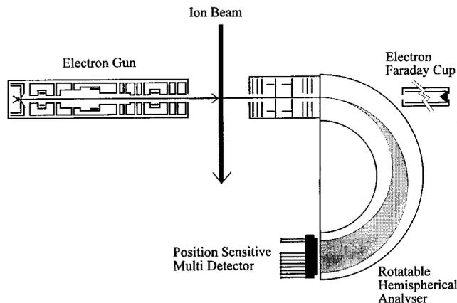
FIG. 1. Schematic diagram of the electron spectrometer.
