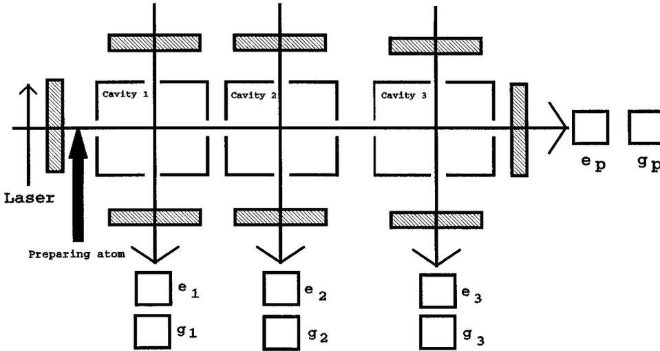
FIG. 1. Proposed experimental setup for preparing and detecting a GHZ state. Three identical cavities are prepared in coherent states by classical sources (not shown). The preparing atom passes through all three cavities. The atoms 1, 2, and 3 are for measuring the parity of the cavity fields. The small squares represent ionization detectors and the shaded regions the Ramsey zones.
