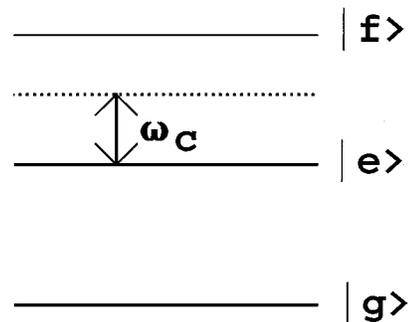
FIG. 2. Rydberg-atom energy-level diagram. The “ground” state  $|g\rangle$  corresponds to a circular Rydberg state of principal quantum number  $n=50$ , and  $|e\rangle$  corresponds to  $n=51$ .
