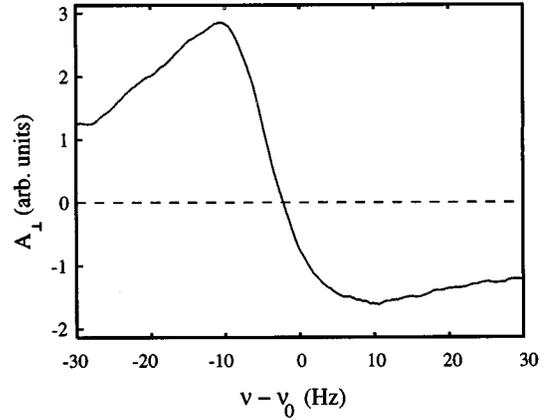
FIG. 5. Spectrum of magnetic resonance obtained by monitoring the transmitted light intensity.
