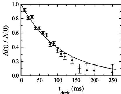
FIG. 2. FID amplitude as a function of the duration of the dark period. The solid line is a fitted single exponential.
