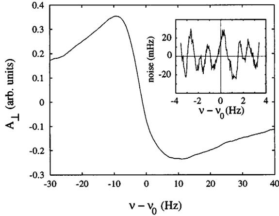
FIG. 4. Magnetic resonance spectrum recorded with LIF detection by scanning the driving radio frequency  $\nu$  over the resonance at  $\nu_0 \approx 40$  kHz (lock-in time constant 30 ms). The digital integration time was 1 s per sampling point. The inset shows the residuals of a fit with a fifth-order polynomial as discussed in the text.
