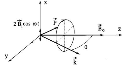
FIG. 3.  $B$ -field geometry in the driven precession experiments.
