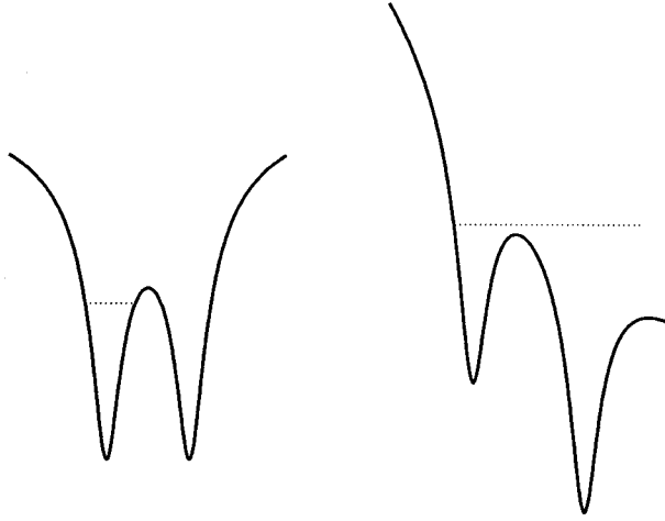
FIG. 1. Schematic molecular ion potentials without (left) and with (right) the applied laser field. An electron occupies the left well, while the right well has a net positive charge. The internuclear barrier is lowered by the positive charge of the right well and so at a certain internuclear distance the electron is able to tunnel through the barrier and escape the molecule.
