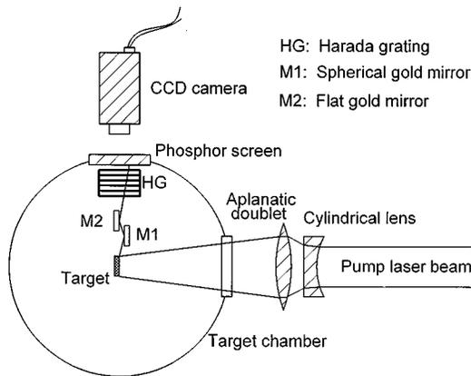
FIG. 1. Setup of the target chamber, the focusing optics, and the x-ray diagnostics used for the measurements.
