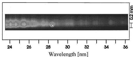
FIG. 2. One-dimensional space-resolved spectrum for a 2.4-cm-long chromium target. For this shot a 0.7% prepulse was used and the energy of the main pulse was 82 J. The  $J=0-1$  lasing line at 28.5 nm is observed to dominate the spectrum. The wavelength axis is in the horizontal direction and covers the spectral region between 23 and 35 nm.
