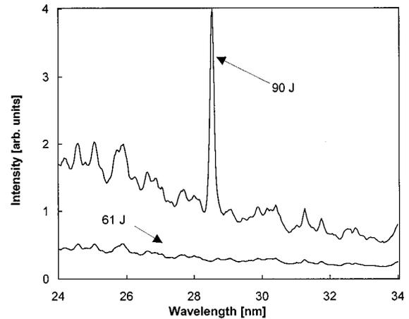
FIG. 3. Spectral scans along the wavelength axis for two different main pulse energies and a 0.7% prepulse.
