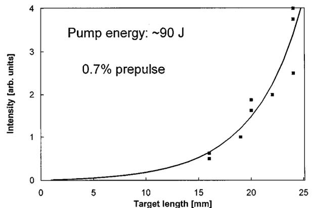
FIG. 4. Lasing intensities for the  $J=0-1$  lasing line at 28.5 nm as a function of the target length for a drive laser energy of  $90 \pm 5 \text{ J}$  and a 0.7% prepulse. A least-squares fit to the Linford-formula [27] yields a gain coefficient of  $2.2 \pm 0.5 \text{ cm}^{-1}$  and is shown as a solid line.
