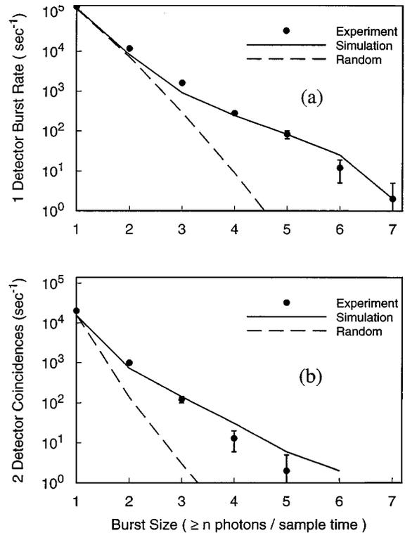
FIG. 3. Experimental and theoretical burst and coincidence distributions on the  $^{26}\text{Mg}^+$  resonance: (a) burst signal from a single detector and (b) delayed coincidence signal using two detectors. The random statistics line (dashed) in (a) is a Poisson distribution using the average count rate, while in (b), it is the expected rate of random coincidences based on the measured rate of bursts in each detector.
