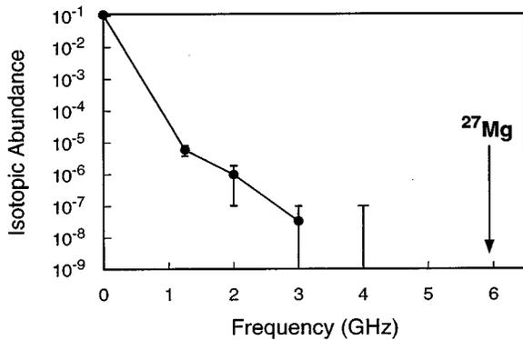
FIG. 2. Isotopic abundance sensitivity as a function of detuning from the  $^{26}\text{Mg}^+$  resonance. The vertical axis represents the background coincidence rate at clip level 4, measured at different detunings from the  $^{26}\text{Mg}^+$  resonance, normalized to the on-resonance signal and scaled by the abundance of  $^{26}\text{Mg}$ .
