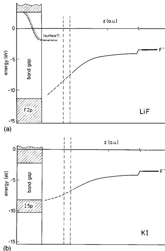
FIG. 3. (a) Energy diagram for the affinity level of a  $\text{F}^-$  ion in front of a LiF surface. The vertical dashed lines indicate a typical range of distances of closest approach of the projectiles to the surface. (b) Energy diagram for the affinity level of a  $\text{F}^-$  ion in front of a KI surface.
