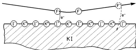
FIG. 2. Sketch of a trajectory of fluorine atoms scattered from a KI monocrystalline surface. Electron capture proceeds from  $\text{I}^-$  bound to lattice sites of the alkali halide crystal.
