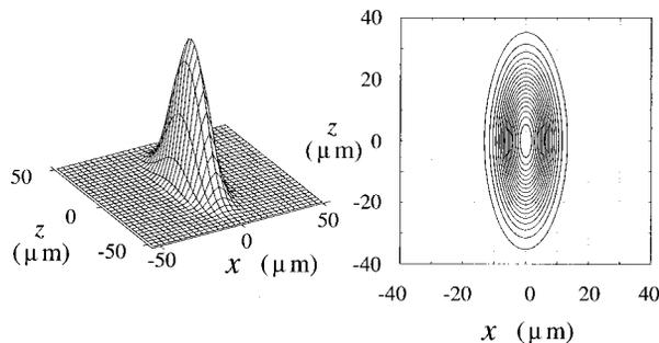
FIG. 2. The evolved density distribution  $\mathcal{F}(x,z)$  found by evaluating the self-consistent wave function for 2000 atoms, abruptly reducing the spring constants for the harmonic potential, and expanding for 60 ms.
