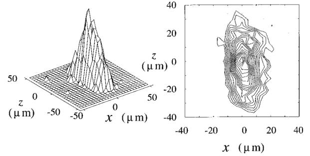
FIG. 3. The experimental image of the rubidium condensate observed on the camera after an expansion time of 60 ms.
