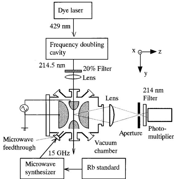
FIG. 2. Experimental setup. Helmholtz coils for compensation of the magnetic field are not shown here for simplicity.
