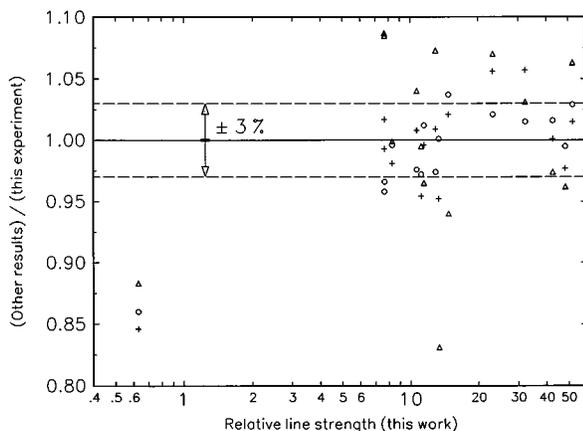
FIG. 1. Comparison of our measured line strengths, normalized within each multiplet to 100, with line strengths according to  $LS$  coupling (triangles) and the intermediate coupling data of Ref. [2] (pluses) and Ref. [4] (circles) for lines within  $3s$ - $3p$  triplets. We show an error band of  $\pm 3\%$  (broken lines), since our experimental uncertainties lie in the range from  $\pm 2.6\%$  to  $\pm 3\%$  for all but the weakest line (where the uncertainty is  $\pm 5\%$ ).
