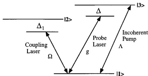
FIG. 1. V-type three-state system for lasing without population inversion.
