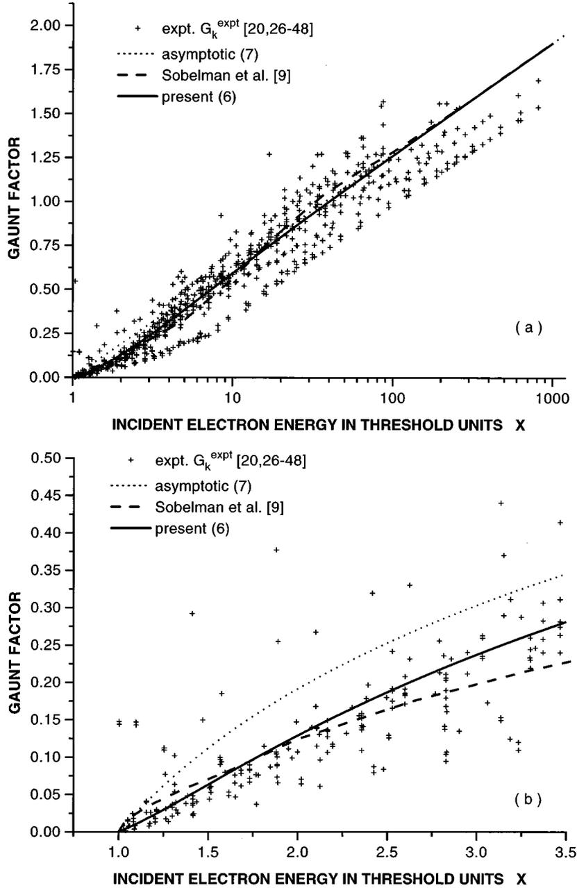
FIG. 3. (a) Gaunt factor for allowed transitions with  $\Delta n > 0$  in atoms with  $LS$  coupling. The values  $G_k^{\text{expt}}$  are inferred from experimental cross sections (listed in Table II) using the Van Regemorter formula. (b) Fragment of (a).
