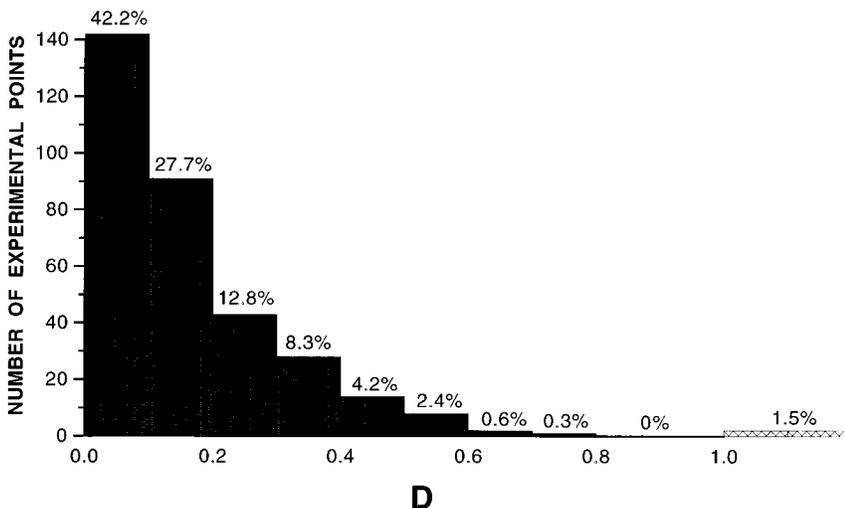
FIG. 2. Distribution of experimental values  $G_k^{\text{expt}}$  presented in Fig. 1(a) over their deviation from the Gaunt factor (4): numbers of  $G_k^{\text{expt}}$  per 10% intervals of deviation (5).
