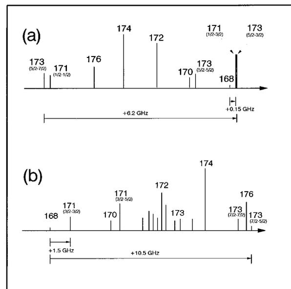
FIG. 7. The absorption spectra of ytterbium (a) for the first transition line:  $6s^2 1S_0 - 6s6p^3 P_1$  and (b) for the second transition line:  $6s6p^3 P_1 - 4f^{13} 6s^2 6p^3 (\frac{7}{2}, \frac{3}{2})_2$ .
