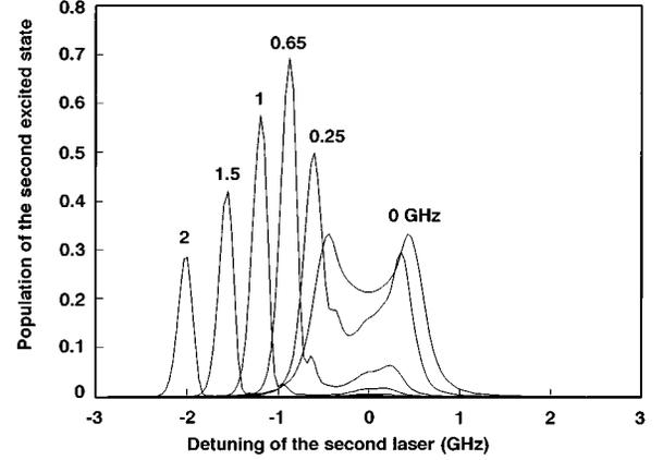
FIG. 2. Numerical results for the population of the second excited state. The detuning of the first laser was fixed at 0, 0.25, 0.65, 1, 1.5, and 2 GHz while the detuning of the second laser was scanned.
