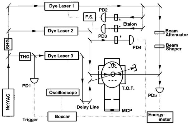
FIG. 3. Schematic diagram of the experimental setup. (SHG: second-harmonic generation; THG: third-harmonic generation; F.S.: frequency stabilizer; PD: photodetectors; MCP: microchannel plate; T.O.F.: time-of-flight mass spectrometer).
