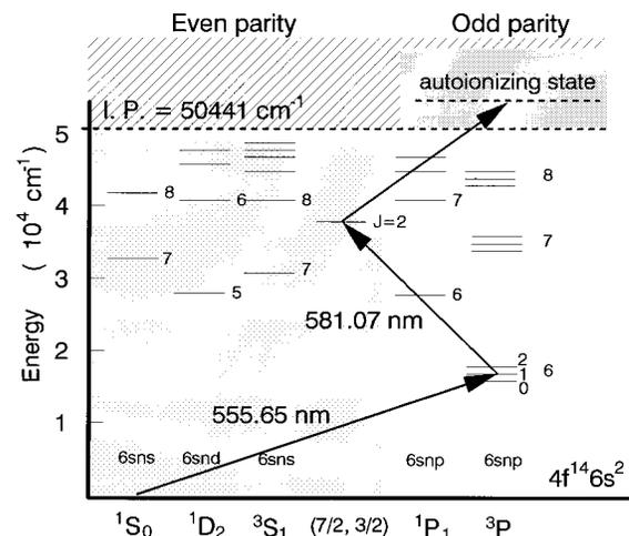
FIG. 1. Energy-level diagram and photoionization scheme of ytterbium. I.P. denotes the ionization potential.
