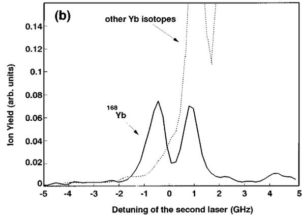
FIG. 4. Experimental ion yields of  $^{168}\text{Yb}$  and other Yb isotopes as a function of the detuning of the second laser when the detuning of the first laser was fixed (a) at 0.65 GHz and (b) at 0 GHz.
