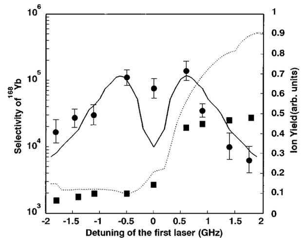
FIG. 6. Experimental and numerical results for the selectivity and ion yield of  $^{168}\text{Yb}$  as a function of the detuning of the first laser. —: ion yield (numerical), ●: ion yield (experimental), ·····: selectivity (numerical), ■: selectivity (experimental).
