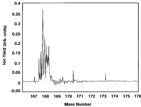
FIG. 5. Mass spectrum of Yb ions detected by MCP and oscilloscope when the ion yield of  $^{168}\text{Yb}$  was maximum in Fig. 4(a).
