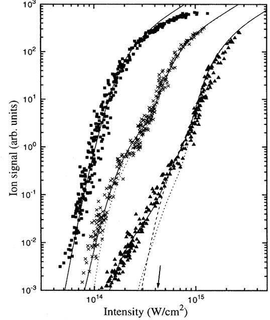
FIG. 1. Argon-ion signal as a function of incident laser intensity for a 600-fs 1053-nm linearly polarized laser pulse. Each point represents a single laser shot. The calculated curves are shown as dotted lines (ADK plus electron rescattering model), solid lines (ADK plus curve fit for NS double and triple ionization), and dashed lines (ADK plus curve fit for NS double ionization only). The experimentally measured intensities are multiplied by 1.2 for comparison to the calculations.
