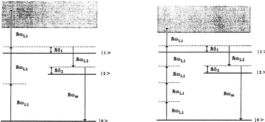
FIG. 1. Energy-level diagram defining detunings for various transitions.
