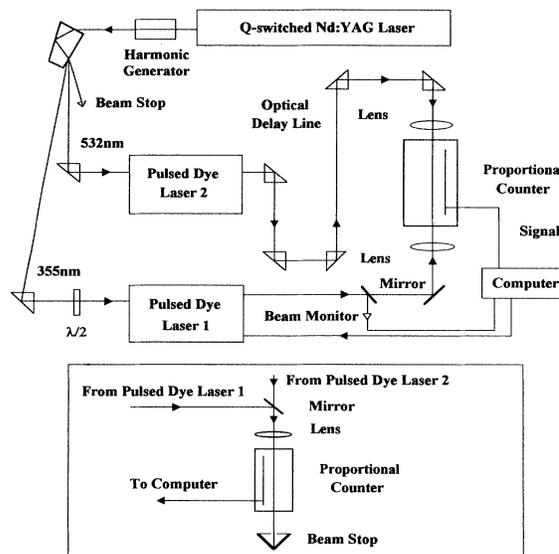
FIG. 3. Experimental setup for studying the ac Stark shifting of two- and four-photon resonances. Inset: setup for copropagating-beam configuration.
