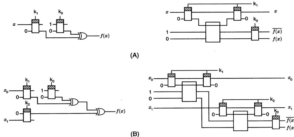
FIG. 3. Boolean logic (left) and reversible logic (right) circuits for the calculation of the (a) one-bit and (b) two-bit functions  $f(x)$ .  $k_0, k_1,$  and  $k_2$  control the classical switches which determine the function calculated. They are set (secretly) by Bob.
