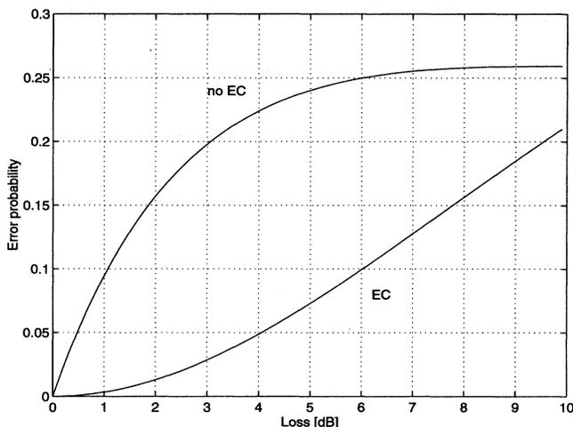
FIG. 6. Error probability for the final measurement result in the  $k_1, k_0 = 10$  case, with and without error correction (lower and upper curves). As loss increases to infinity, the error correction scheme becomes ineffective because the photons become localized in an arm of the interferometer, but for small  $\gamma$ , the improvement is substantial;  $P_{\text{NEC}} \sim \gamma/2$  and  $P_{\text{EC}} \sim \gamma^2/16$ , where loss is  $4.34\gamma$  dB.
