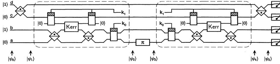
FIG. 4. Complete quantum computer system used to solve the one-bit Deutsch problem. The apparatus in the dashed box is used by Bob to calculate  $f_k(x)$ , and everything else belongs to Alice. In principle, it is not necessary to send mode  $d$  to Bob, although it may simplify the implementation in practice.
