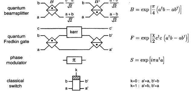
FIG. 2. Unitary transforms for the components of our quantum computer. The operators  $a$  and  $a^\dagger$  are the usual annihilation and creation operators.
