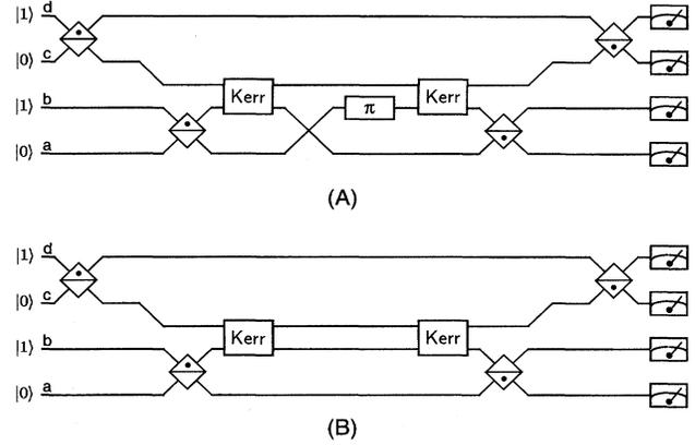
FIG. 5. Simplified versions of the quantum computer circuit when  $k_1k_0=10$ , Bob's apparatus is merged in, and (a) the  $\pi$  phase shift  $S$  is in place, or (b)  $S$  is removed.
