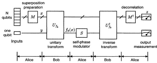
FIG. 1. Algorithm for solving Deutsch's problem using a quantum computer.
