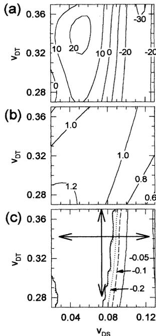
FIG. 2. Calculated frequency shifts for a  $^{135}\text{Cs}$  fountain in mHz for an average density of  $10^9 \text{ cm}^{-3}$  and a launch temperature of 2.6  $\mu\text{K}$ . (a) Frequency shift caused by the  $F=3, m_F=0$  state versus  $v_{DS}$  and  $v_{DT}$ . (b) Shifts caused by the  $F=4, m_F=0$  state. (c) The ratio of the shifts in (a) and (b). The arrows denote the likely ranges of  $v_{DS}$  and  $v_{DT}$  for  $^{135}\text{Cs}$ .
