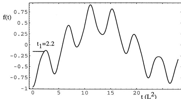
FIG. 2. The time dependence of the center of the wave packet Eq. (5.16) for the period  $10\pi/(E_1 - E_0)$ . Only the part shown in the interval  $0 \leq t \leq 2.2(L^2)$  is used to test Prony's inversion. Thus if  $f(t)$  is known accurately in this interval then the complete curve can be constructed.
