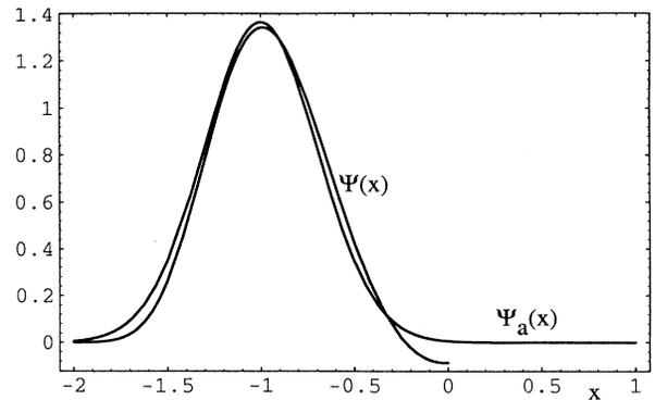
FIG. 1. The exact Gaussian wave packet  $\Psi_g(x)$  and its approximate form  $\Psi_a(x)$  obtained from the superposition of four eigenstates, Eqs. (5.2)–(5.6).
