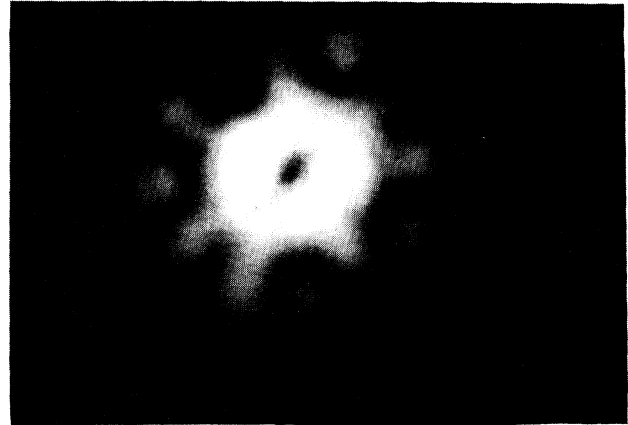
FIG. 12. Simultaneous emission of a q = 1 "doughnut mode" and a pattern of the q = 6 mode family.
