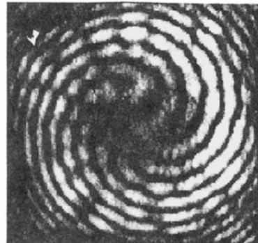
FIG. 5. Pattern with nine phase singularities (vortices): (a) intensity and (b) "spiral" interferogram of pattern with charge-9 phase singularity.
